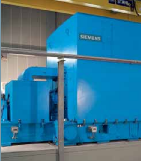
35-MW motor running at 5,040 rpm for a compressor station of a gas pipeline from Great Britain to Belgium
