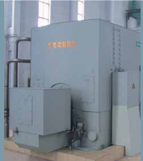
42-MW motor for the blast furnace blower in the Anshan steelworks, China
