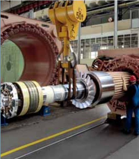
65-MW compressor motor running at 3,600 rpm for the first completely electric gas liquefaction system in the world in Hammerfest/Norway
