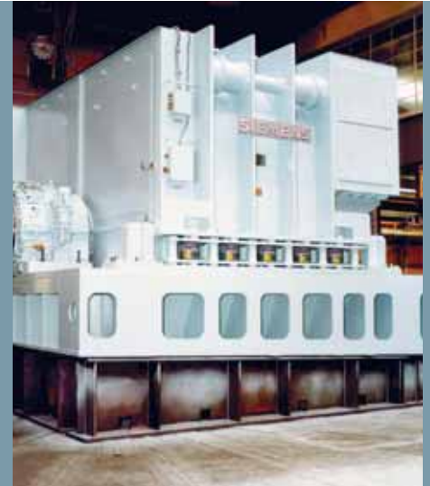
One of the two 21-MW motors for the main drive of a cruise ship
